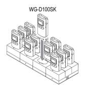
Step**5**: LEDs on the charger fast flash 5 times (approx. 5 seconds) indicates synchronization is talking place
