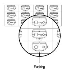
Step**6**: LEDs turn to solid and now indicate the battery charging status. The synchronization process is completed and you are ready to use your system.
